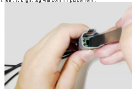
3.推动端子垂直插入连接器内，听到一声清脆的喀嚓声表明端子插接到位。 Push contact straight into connector until a 'click' is felt . A slight tug will confirm placement .
