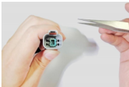
5.将压板放到连接器内。 Put the wedge into connector with tweezer .
