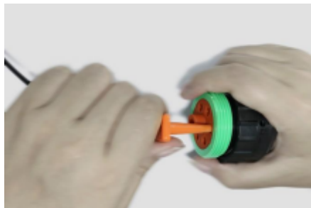
2. 将工具插入连接器后部的孔中，直到感觉到阻力为止。 Slide tool along the wire into the insert cavity until it engages contact and resistance is felt .
