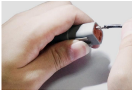
2.抓住芯线将端子对正连接器的相应孔位。 Hold connector with rear and insert contact depending on corresponding hole .
