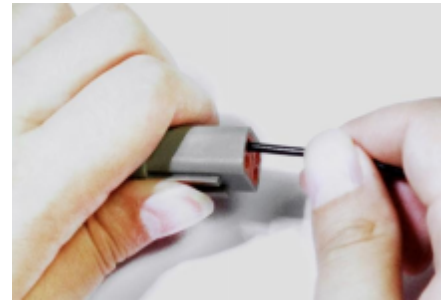
3.推动端子垂直插入连接器内，听到一声清脆的喀嚓声表明端子插接到位。 Push contact straight into connector until a 'click' is felt . A slight tug will confirm placement .
