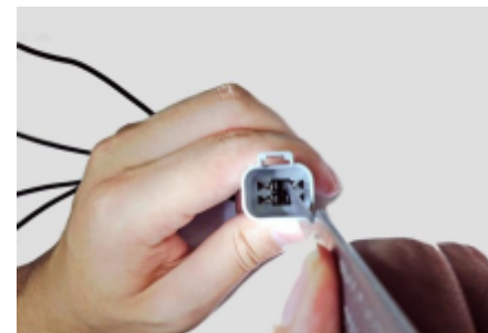
3.用取卸工具的末端把连接器的卡扣撑开，取出端子。 Use the same end of extraction tool to expand the slot and extract contacts from connector.
